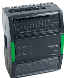
DO-FC-8, DO-FC-8-H 8 Channel Digital Output, Form-C
